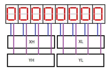
Of each display, 4 segments are connected to the X register, and the other 3 segments are connected to the Y register. Note that each display is connected to the corresponding nibble.
