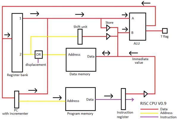
The register bank has one write port (at the left side) and two read ports (at the right side). The output of the ALU can only go to the PC or to one of the registers. A register can be stored in memory through the "Store" buffer.
